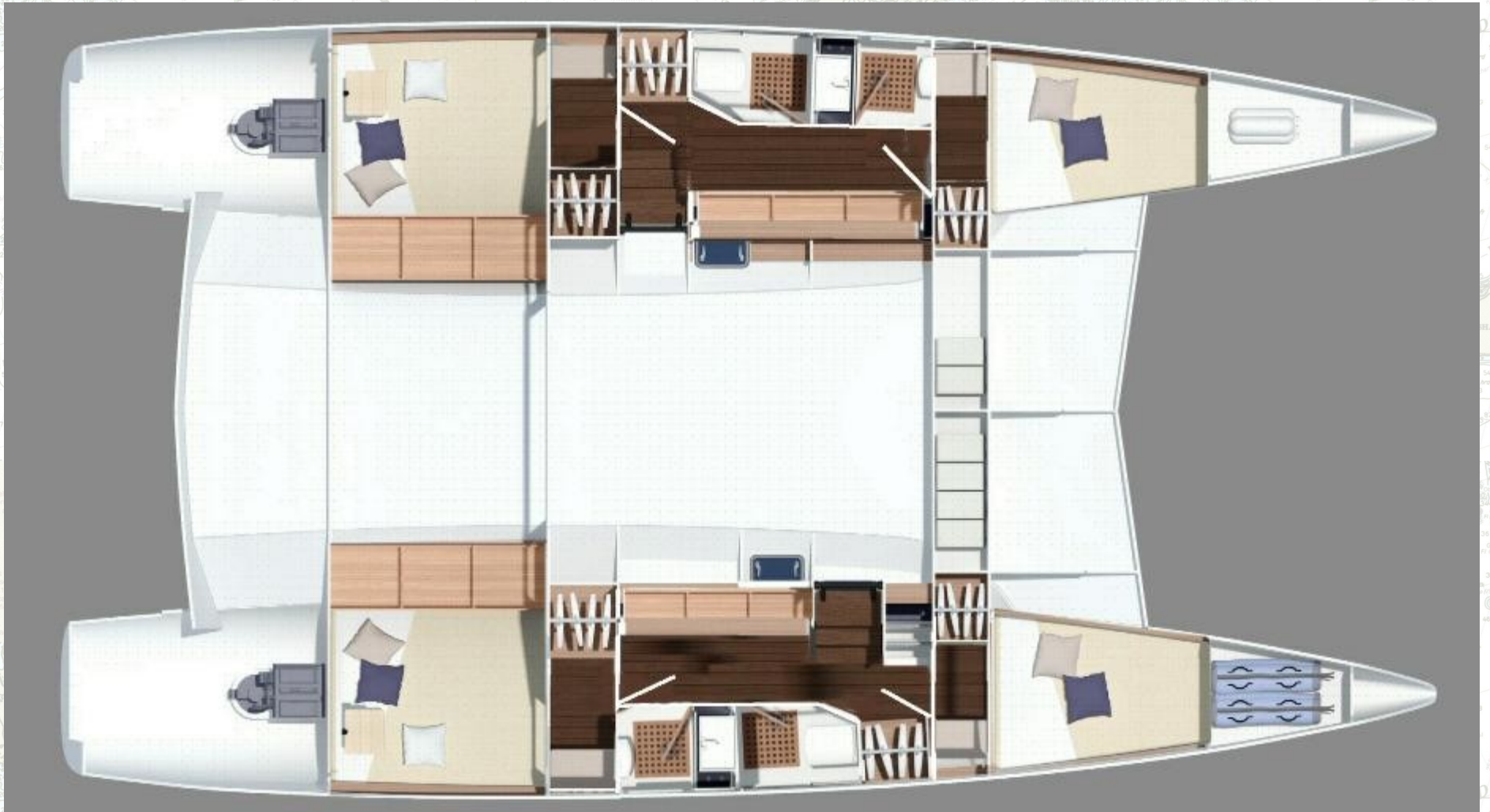
The Alpha 42 Charter Version which features 4 double cabins with 2 separate showers and 2 separate heads.
